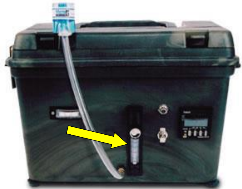
Battery operated sampling pump with built in rotameter
